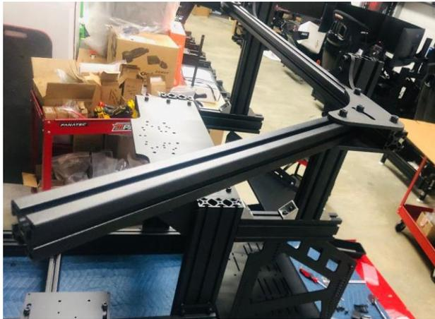
Insert (4) T-Nuts, in the side arm; (2) t-nuts on top and (2) t-nuts on bottom. Position the side arm inside the (2) previously mounted swivel brackets and use (4) M8x16 SHCS and (4) washers to attach (2) Swivel Brackets on the top and bottom. Check to make sure that the swivel cutout is will allow side arms to pivot.
